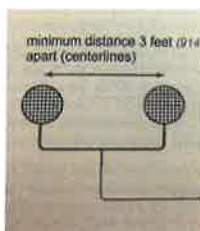
Properly installed suction outlet spacing
